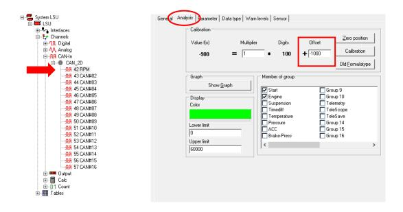
We recommend it to set this up so that heating starts above 1000 RPM, so the battery is not drained when the engine is not running.
