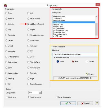
In this example the selected min/max table "Engine" will be exported as an Excel export (marked in red) and it is saved within the temporary directory. The export file name will consist of the event name and the measurement's name (marked in orange). Confirm with **<OK**>.
