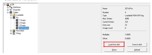
Select table 2DTrkPos, click on button <**Load from disk**>, go to the directory where the tables 2DTrkPos and 2DTrkNme are saved to in the previous step and load 2DTrkPos.
