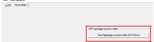
Select tab *Send tables*, click on button **Send laptrigger position table (2DTrkPos)**, go to the directory where the tables *2DTrkPos* and *2DTrkNme* are saved to in the previous step and load *2DTrkPos*.
