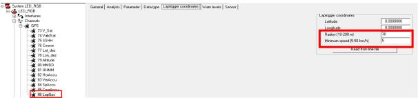
The defined search radius must be large enough to accommodate different driving lines as well as GPS drift. However, if the search radius is too large it may be possible to generate invalid lap times due to the lap signal occurring more than once in a lap, see figure below!
