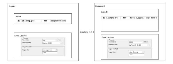
Now the throttle grip of the bike can be used to trigger the Laptimes event, and the dashboard can be used to check if laptime is created correctly.
