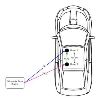
Under real urban driving conditions without houses, trees and bridges 2D RTK system is able to determine the distance between two GNSS modules (rovers) with an accuracy of base line of almost +/- 1 cm up to a speed of 300 km/h.
