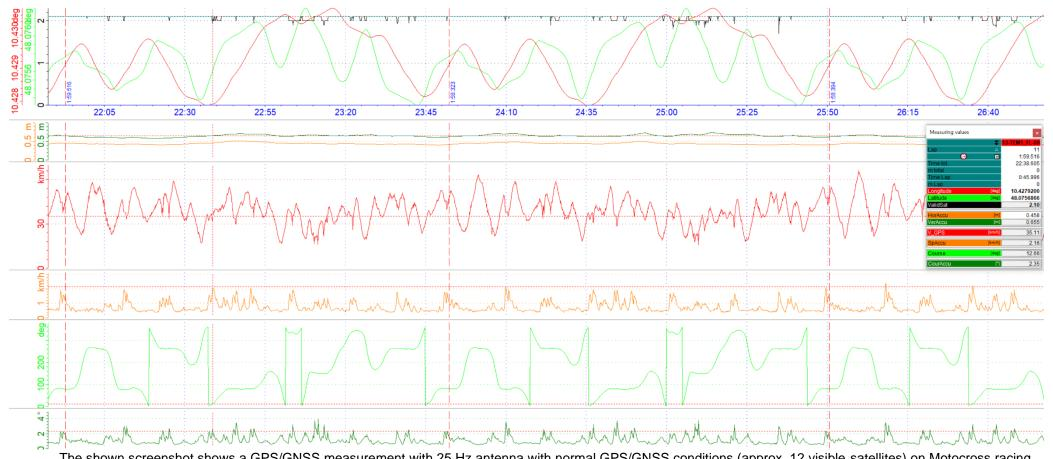
The shown screenshot shows a GPS/GNSS measurement with 25 Hz antenna with normal GPS/GNSS conditions (approx. 12 visible satellites) on Motocross racing track with lap by lap repetition of "accuracy" events by trees or buildings. All accuracies are within the usual limits!
