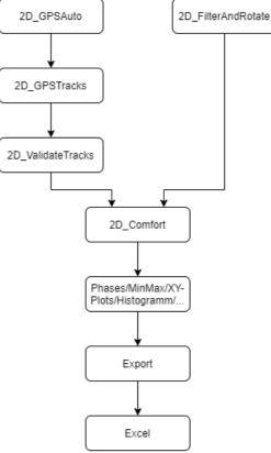
Then the combination of GPSTrack channels provided via the 2D\_ValidateTracks toolchain and the 2D\_Comfort toolchain can be used to calculate the comfort parameters RMS, VDV and MOV.
