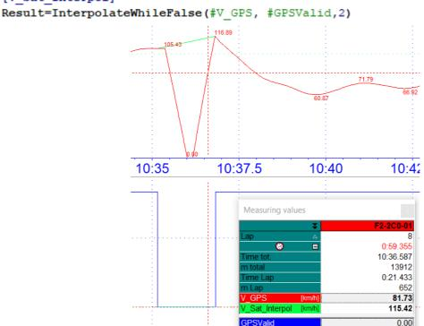
The corrected, green channel #V\_Sat\_Interpol interpolates the signal at the 1.67 second drop of #GPS\_Valid.
