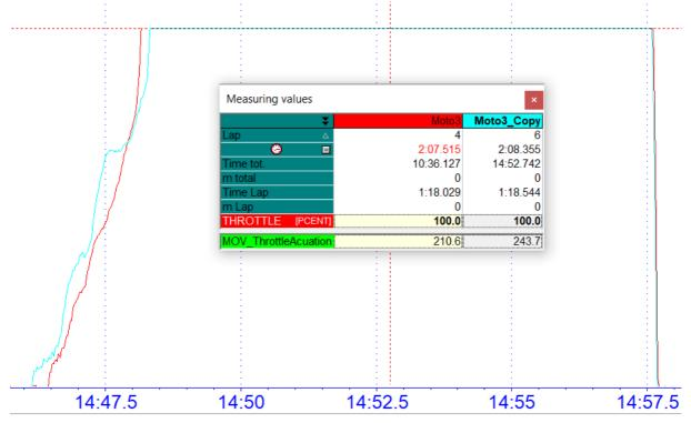
The red measurement Moto3 shows a position of the fastest lap, while the blue measurement Moto3\_Copy shows the same position in the following lap. In the fastest lap the driver has opened the throttle very definitely, while in the following lap the throttle was even closed a little bit during the acceleration phase.
