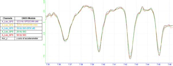
By eliminating the time delay and filtering the coloured longitudinal acceleration channels are compared to the black acceleration signal which shows the actual acceleration of the car at braking and accelerating tests.
