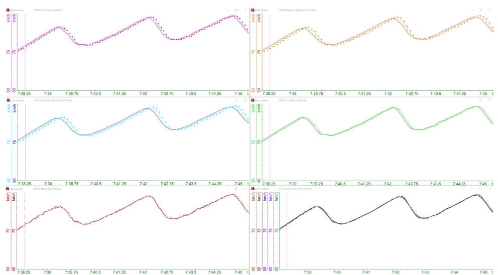
After filtering the raw values in the previous step, the time delay correction mentioned above is now applied. In post-processing, all GNSS channels are shifted to 1/1000 sec with the respective values entered and thus aligned with each other and the actual car movements.
