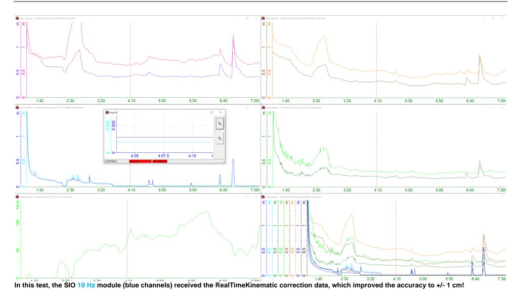
The 50 Hz module is the only module that does not provide any accuracy channels! The remaining modules are not capable of processing RTK correction data. However, the 25 Hz module is superior to the 10 and 12.5 Hz modules in terms of positional accuracy.
