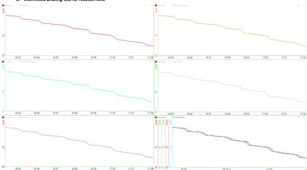
In this test, the driver briefly steps on the brake pedal to brake only briefly at a time in order to make the respective braking processes visible on the unfiltered speed signals shown below.
