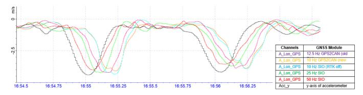
To visualize the time delay and show the differences at modules with various GNSS rates a test was executed where an accelerometer (black channel) was used to compare the actual deceleration of the car by accelerometer with the derivation of the speed signals (longitudinal acceleration) at the braking tests from previous chapter.
