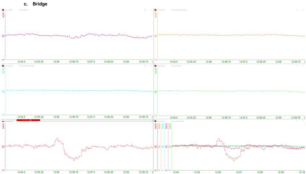
The behaviour of the different GNSS modules in this test strongly depends on how many GNSS satellites are used. Since the 12.5 Hz and 50 Hz GNSS module only uses approx. 8 GPS satellites, its behaviour is worst with bridges or trees!
