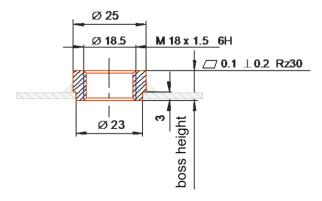
Thread boss dimensions should be as shown in the figure above.
