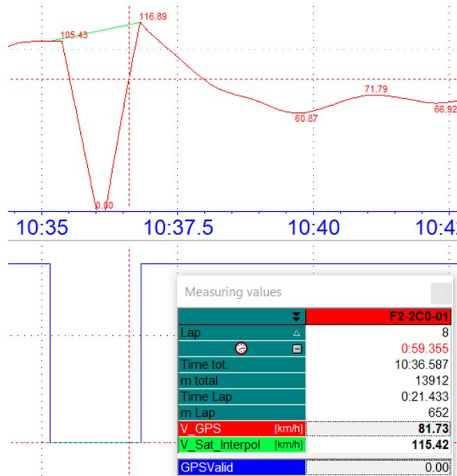
The corrected, green channel #V\_Sat\_Interpol interpolates the signal at the 1.67 second drop of #GPS\_Valid.
